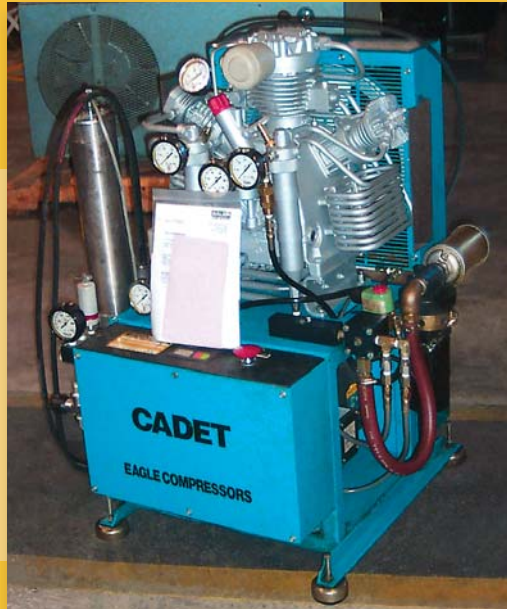
Right: After Re-Blocking Stationary Unit.
